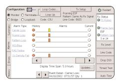
The YBT1 allows users to gather detail on any of the alarm or error events. Simply touch any of the red events and the instrument provides detail about the network event. This detail includes the number of events and the time of the event, and provides useful information to correlate network logs to field data.
