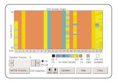
The DSO Activity Graph arranges the DSOs into columns. Time is the vertical axis and different densities are shown with different colors. With this unique feature, users can quickly verify the presence of traffic, signaling channels, etc. and how the data is changing over time.
